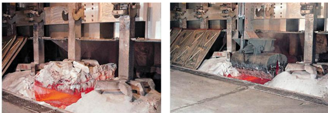
Figure 3. Anode change in a conventional cell.
